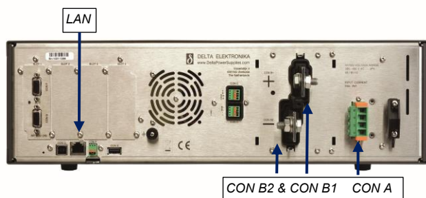
Figure 5.2: Connections on the rear side
