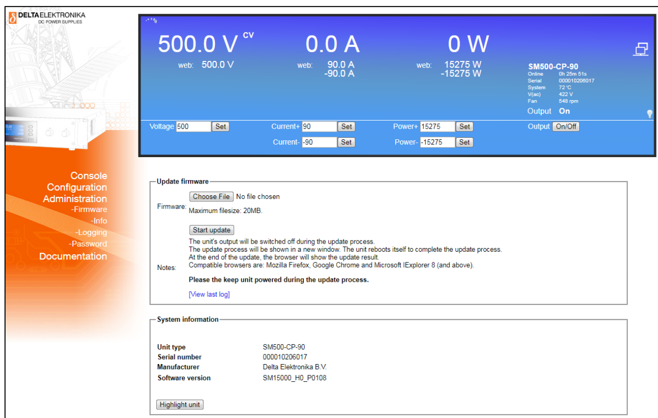
Figure 8.3: Via the web interface the downloaded firmware package can be uploaded to the unit.
