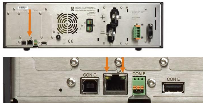
Figure 2.1: Ethernet connector at the rear side
