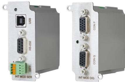
Figure 9.6: Left: Serial programming, Right: Digital I/O
