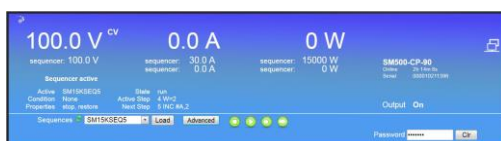
Figure 9.2: Sequencer console for selecting and controlling sequences.
