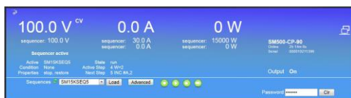
Figure 9.2: Sequencer console for selecting and controlling sequences.
