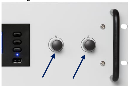
Figure 6.2: Encoders for voltage and current settings
