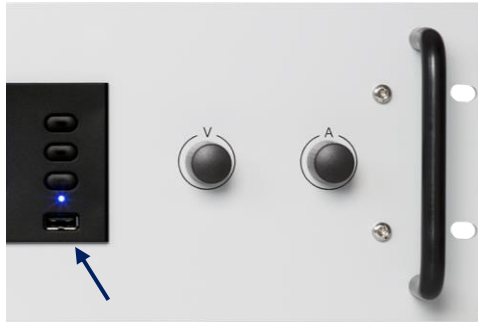
Figure 7.7: The location of the front USB-connector.
