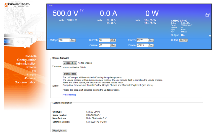
Figure 6.11: Via the web interface the downloaded firmware package can be uploaded to the unit
