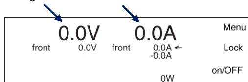
Figure 7.17: The first line in the display shows the actual output value for voltage and current.
