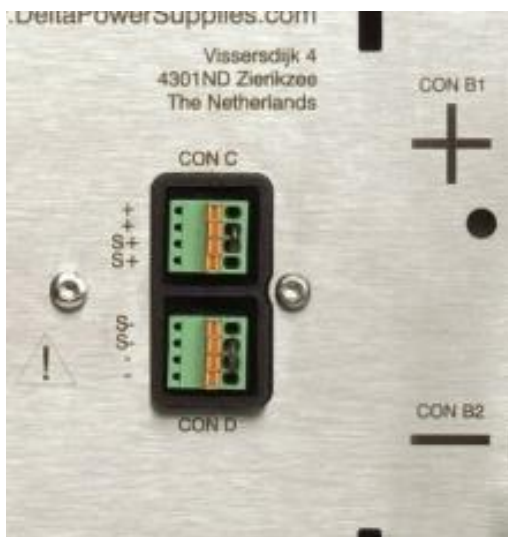
Figure 10.2: For normal operation links should be connected between S+ and +, and between S– and –.
