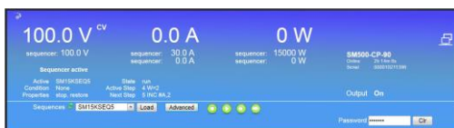
Figure 9.2: Sequencer console for selecting and controlling sequences.
