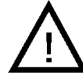
Figure 10.7: If the Internal Error-icon is shown on the display, the DC-power output of the unit will shut down.
