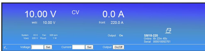
fig 4 - 5 The front console of the web interface for setting of the output and monitoring various parameters.
