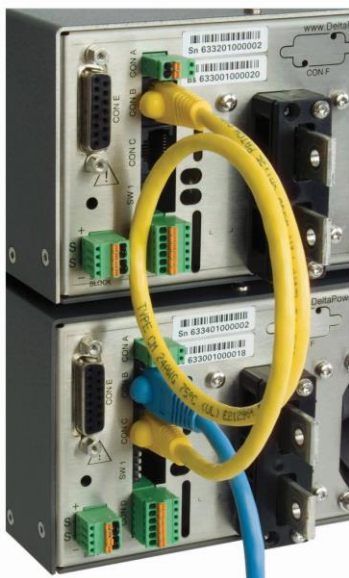
fig 4 - 22 Use standard UTP cables (RJ45) for Master / Slave operation.
