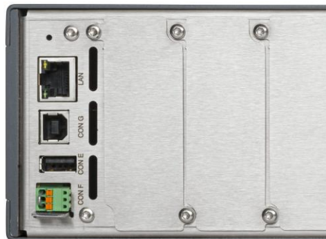
Figure 2.1: Ethernet connector at the rear side
