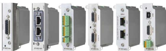
Figure 6.5: Different interface modules can be plugged in.
