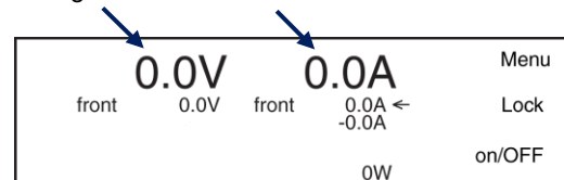
Figure 7.13: The first line in the display shows the actual output value for voltage and current.
