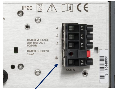
Figure 7.1: Insert the included 4-pole header in CON A for the connection of the AC power / Mains.
