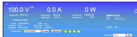
Figure 9.3: Sequencer console for selecting and controlling sequences.
