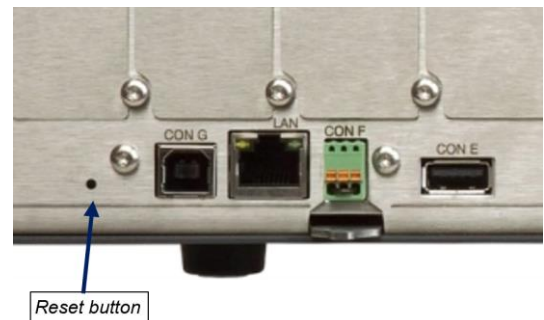
Figure 10.8: Location of the reset button.
